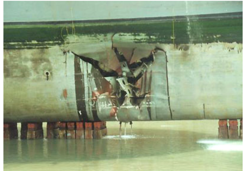
USS Tripoli contact mine damage
